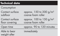
Suitable for indoor use on absorbent and non-absorbent surfaces (walls, floors and ceilings). Also suitable for repair work, bonding on top of inspection covers and other applications.
