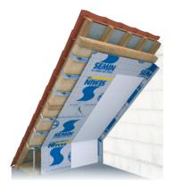
The minimum overlap of the edges is 5 cm, and the edges are joined using Semin universal adhesive tape. When using the vapour barrier with adhesive tape, simply cover each edge by 5 cm and apply the tape ensuring that the latter is properly sealed.
